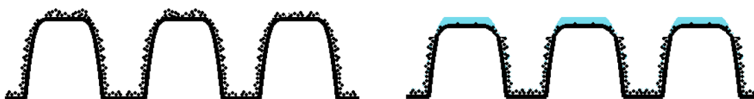
Figure 5. Schematic explanation of the enhanced conductivity of a laser-textured surface of glass after an abrasion test. Before the abrasion test (left), the surface conductivity is extremely low because of the absence of a conductive water layer atop the electro-insulating coating. After the abrasion test (right), the replacement of surface hydrophobic texture by the hydrophilic glass surface is accompanied by the formation of water films on hydrophilic patches (colored blue) in a humid atmosphere. The presence of electro-insulating bridges separating the conductive water layers favors the good electro-insulating performance of superhydrophobic coatings on glass even after the abrasion test.
